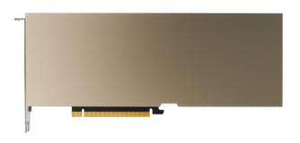
**CUDA Cores** 3804 **Tensor Cores** 224 FP32 Performance 10.3 TFLOPS **GPU Memory** 24 GB HBM2 ECC **GPU Memory Type** Memory Bandwidth 933 GB/s Memory Interface 3072-bit System Interface PCI-E 4.0 x16 Max Power Consumption 165 W Thermal Management Passive
