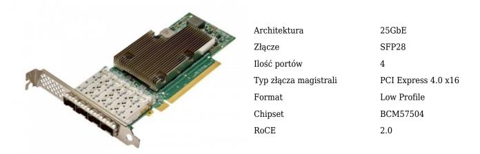
Based on Broadcom's scalable 10/25/50/100/200G Ethernet controller architecture, the P425G 4x25G PCIe NIC is designed to build highly-scalable, feature-rich networking solutions in servers for enterprise and cloud-scale networking and storage applications, including high-performance computing, telco, machine learning, storage disaggregation, and data analytics.
